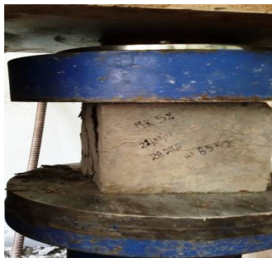
Figure 4: Failure of concrete specimen under CTM
