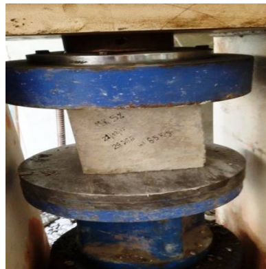
Figure 3: Experimental Setup for compressive Strength test
